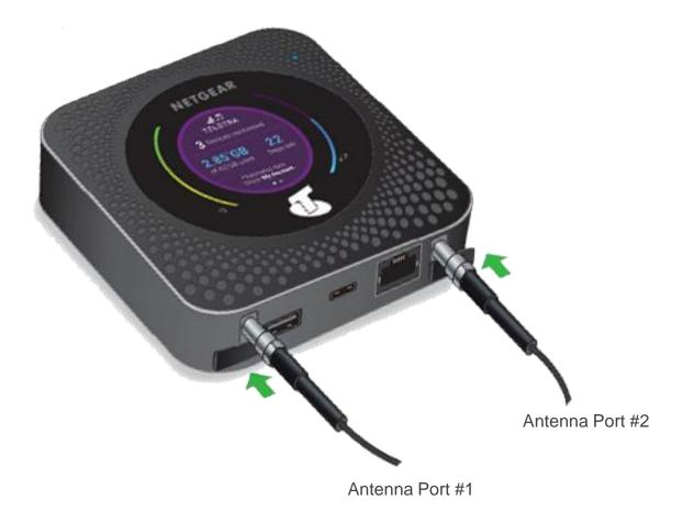
Warning: The AT&T Netgear Nighthawk MR 1100 Router has 2 external antenna port. For single antenna use, either port can be used. Use both ports for MIMO (Dual Antennas) use. Antenna ports can be fragile. Using excessive force when connecting or disconnecting your adapter cable can damaged the modem's internal antenna. To avoid damaging your modem - Be Gentle.
